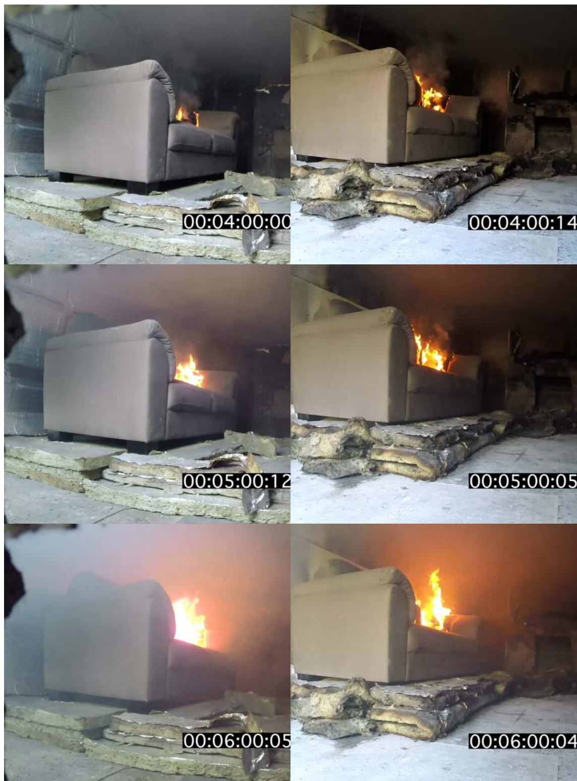
Plate 17 – Image of fire development Exp.07 and Exp.03 (4 to 6 min)
