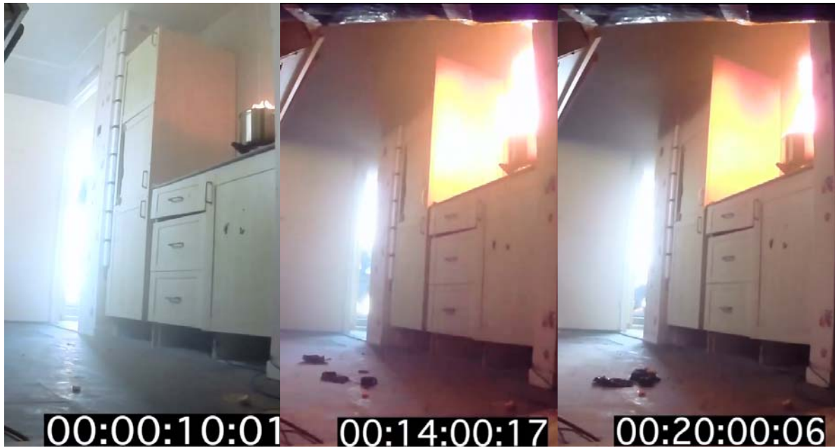
Plate 9 – Images from within the fire compartment for Experiment 01
