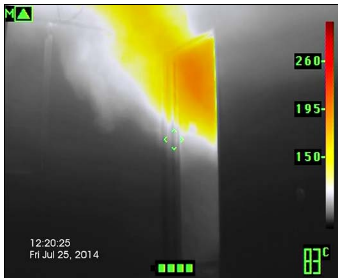
Plate 15 – Image from within the hallway for Experiment 04 (7 min after ignition)
